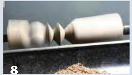
8 A disc shape works well as a transition form from one element to the next, one axis to the next.
