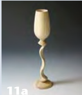
11a The center axis of this multi-axis stem was used to line up the separate components—cup, stem, and base—of this goblet.
