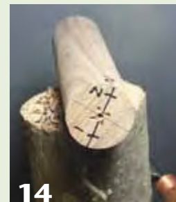
Write the numbers of the axes on the ends and sides of the cylinder so they are clearly visible. Even with a numbering system, though, mistakes are easy to make.
