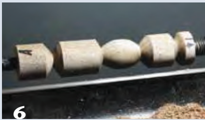
6 Before the end points are changed to create a new axis, a bead and/or V cuts can be made into the cylinder using the initial central axis. Note that the entire spindle is turned to a cylinder before proceeding.
