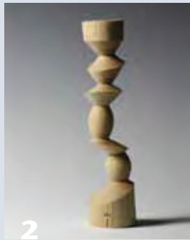
2 This multi-axis spindle is a circular-type multi-axis spindle. There are three axes on the bottom and one center axis on the top.
