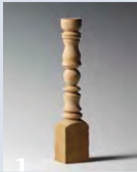
1 This spindle was turned with one central axis. The profile consists of beads, coves, and V cuts.
