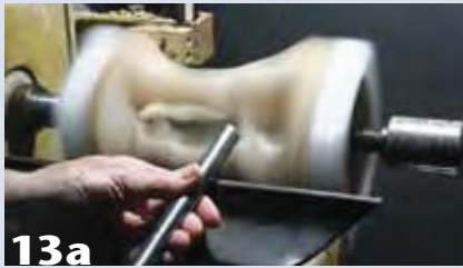
13a Inside-out turnings can be safely held together with strapping tape. In addition, glue is applied at the ends. When finished, all four pieces will have been turned on four different parallel axes.
