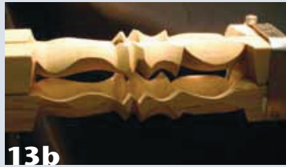
13b These spindles are the result of inside-out turning, turned on all four sides.
