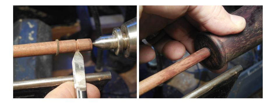
Use repeated shallow cuts and creep up the on fit !!
