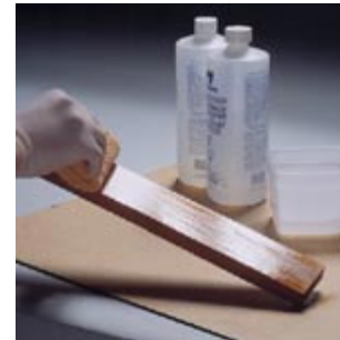
Apply the bleach as evenly as possible, and keep the surface wet as you work.
