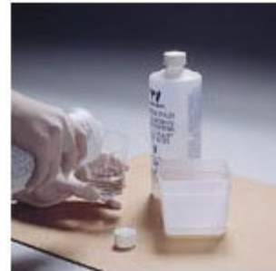
Work fast after mixing the two chemicals. The solution begins to neutralize—and lose bleaching power—just as soon as you start to pour the liquids together.
