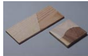
After bleaching, the oak and walnut are the same color. The grain remains visible in both pieces.
