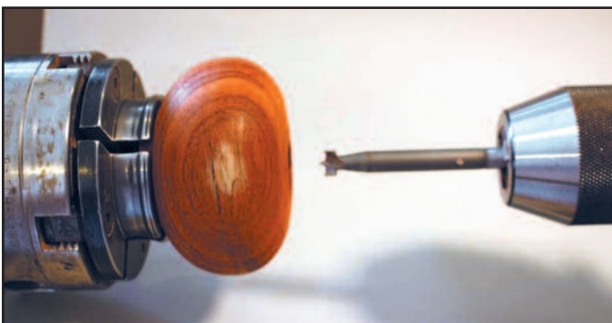
Step 23. Use a 3/8" Forstner bit to drill through the back of the body at the headstock end. Remove the hollowed body from the chuck.
