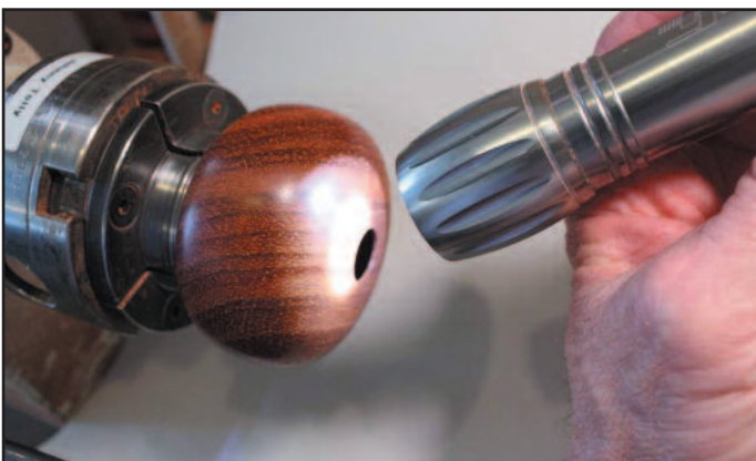
Step 22. I use a small LED flashlight to look in the body while checking for any ridges that may need more attention.
