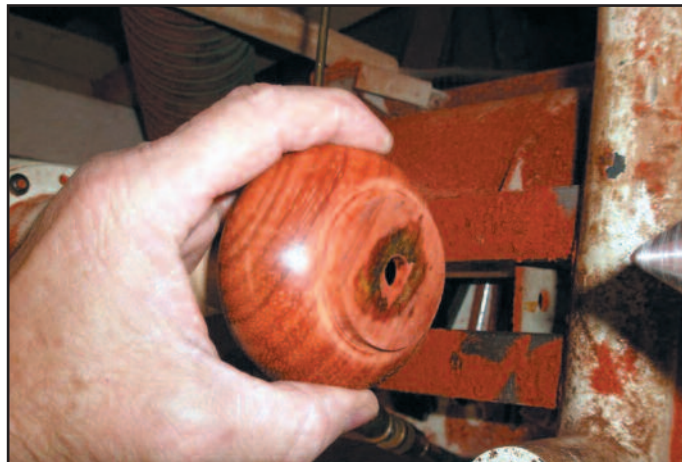
Step 24. The part that was in the Oneway Talon chuck is shown. Note that the wall thickness is about 3/16" in the 3/8" hole. Also note that the CA helped to prevent any splintering of the wood.
