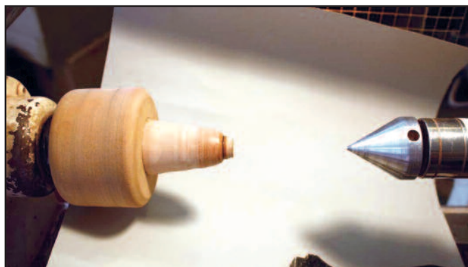
Step 25. If you have not made a friction drive similar to the one shown here, now is the time to do it. The friction drive will hold the ornament body between centers to turn away the small tenon that was used to hold it when hollowing out the body.
