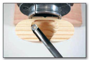
Start by using the *Hunter* 3/8" straight tool. Make a series of cuts starting at the opening and going back until the back of the 5/8" hole is reached.
