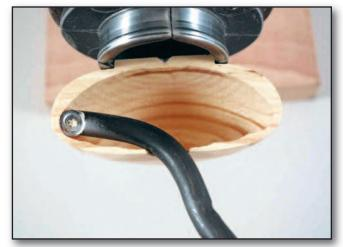
Finally, the 3/8" swan neck tool is used again to make the finishing cuts, cutting from the back of the body to the center. Use a thickness gauge often while working with any of the *Hunter* tools to prevent cutting through the side of the ornament body.
