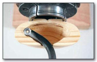
Next, with the *Hunter 3/8*" swan neck tool, make a series of cuts starting at the opening again and going back until the back of the 5/8" hole is reached.
