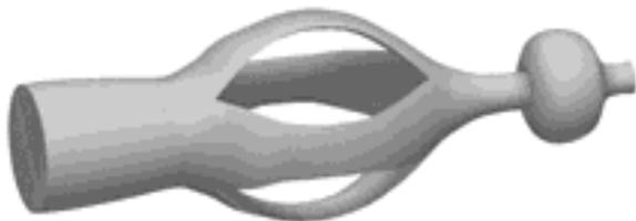
You should get most of the body finish turned before turning down the end towards the headstock, while there is still enough wood to avoid whip and chatter. I don't recommend spin-sanding here, the piece tends to grab and tear the
